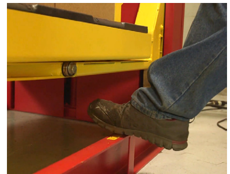
Photo-eye toe sensor protects workers.
