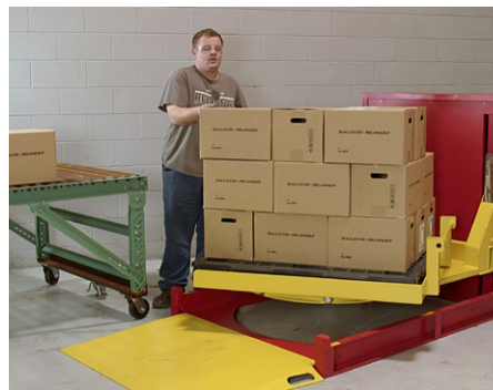
Turntable eliminates walking around the load.
