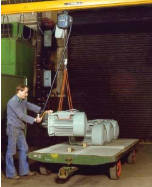
A portable gantry crane fitted with an electric hoist
