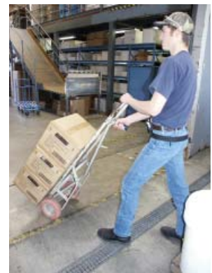
This hand truck has an additional handle to provide better directional control.
