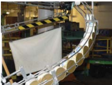
Small containers and lightweight loads can be handled by gravity conveyors.
