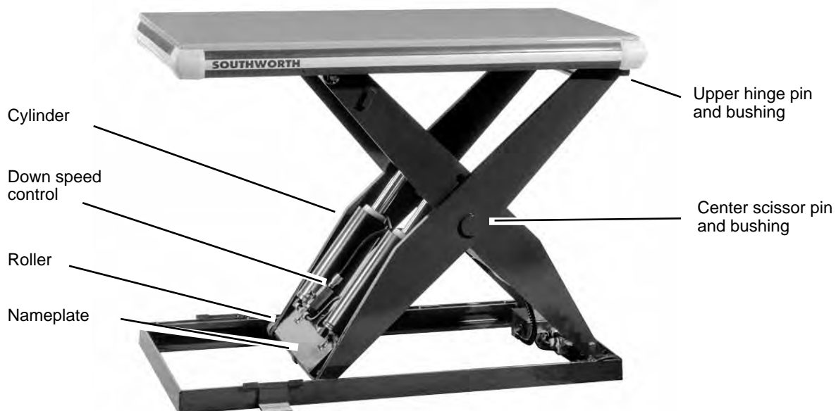
Figure 10 – Parts Identification, Side View
