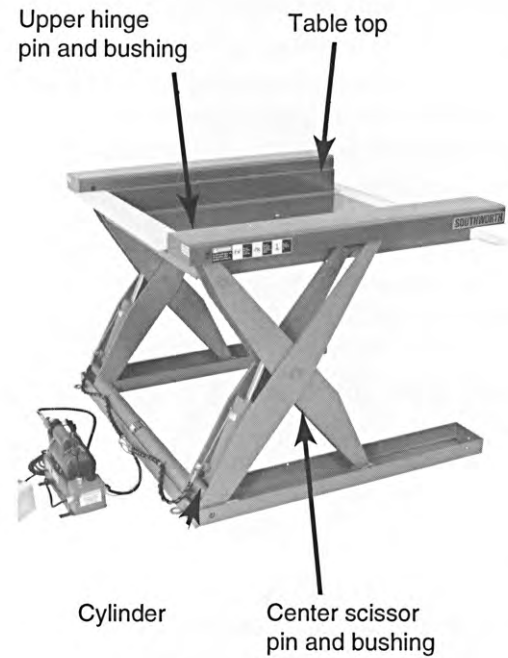
Fig. 9 – Parts Illustration — Rear End of Lift
