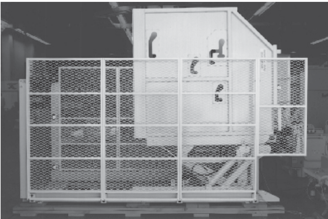
Fig. 2b Operating Sequence - Tilt 90 degree Position
