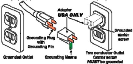
Using an adapter is *forbidden* in Canada. If a grounded outlet is not available, have one installed by a qualified electrician before using this charger.
