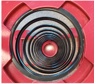
WHITE SPRING IMPROPERLY POSITIONED IN UPPER POCKET
