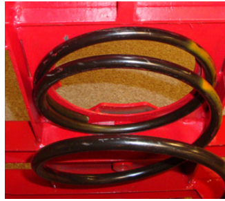
ORANGE SPRING PROPERLY POSITIONED IN UPPER POCKET
