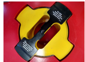
TURN BAYONET 45 DEGREES CCW AND LIFT TO REMOVE
